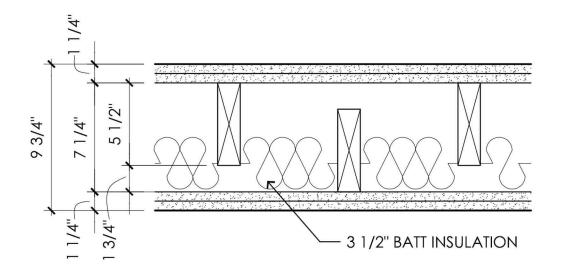
2x6 framing staggered with (2) layers of 5/8" gyp. board applied to both sides. Req'd Fire Rating: 30 mintues (sim. to GA file No. 5530) Sound Rating: 55-58 STC (sim. to NGA 3056)
